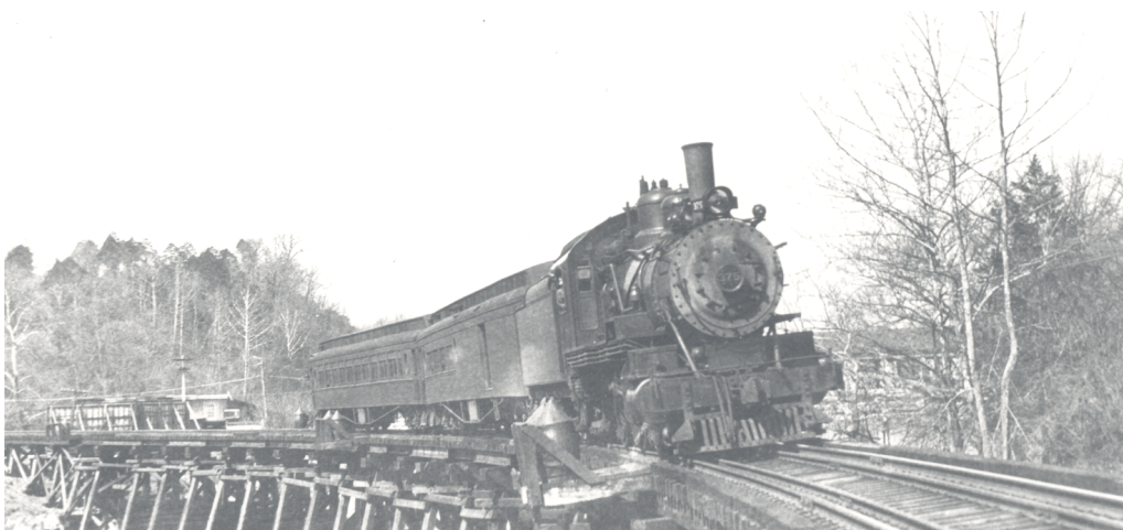
C&O Engine #375, a light 4-6-0 Ten Wheeler, heads a short passenger train across the Maury River toward East Lexington (Photo ca. 1910, APVA, W&L Special Collections).
